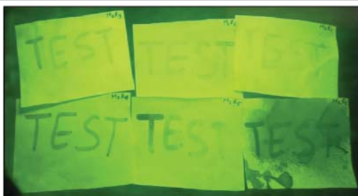
Figure 9: UV Visualization of Ferrous Sulphate on Lime green under UV light.
