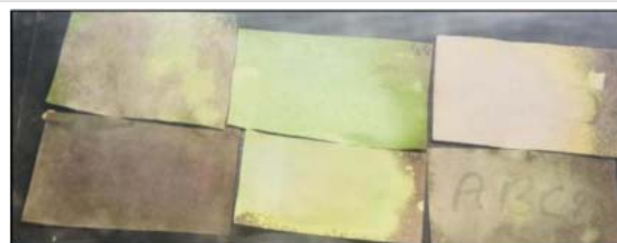
Figure 13: Development of zinc sulphate invisible ink on brown paper under visible light.
